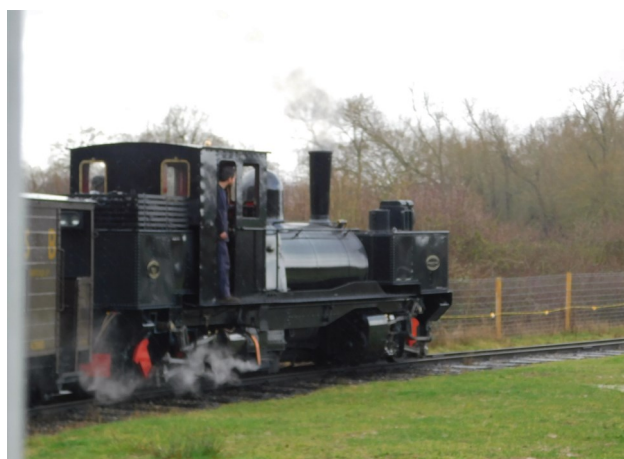
A passing train on the other line, and the loco on the front of ours' - K1 0-4-0T 5292, built by Beyer Peacock in 1909 for Tasmania.
